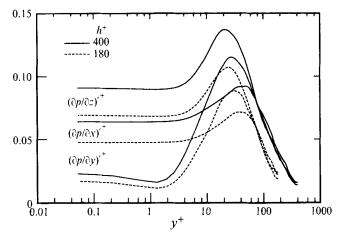
FIGURE 4. Root mean square pressure derivative distributions.
